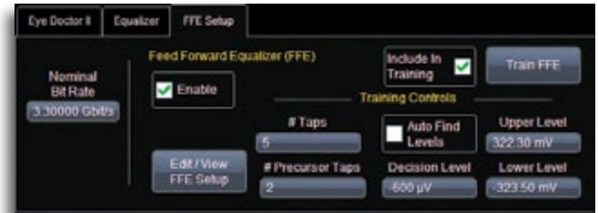
Equalizer and pre/de-emphasis (not shown) are easily modeled via SI Studio's "EyeDoctor II" dialogs.
