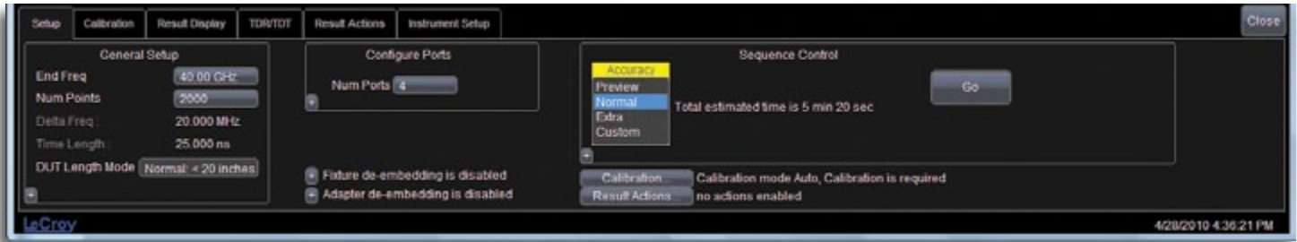
The main SPARQ setup dialog shows all of the information needed to take S-parameter measurements in minutes.
